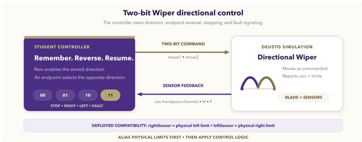
Figure 2. Directional two-bit Wiper control loop.
